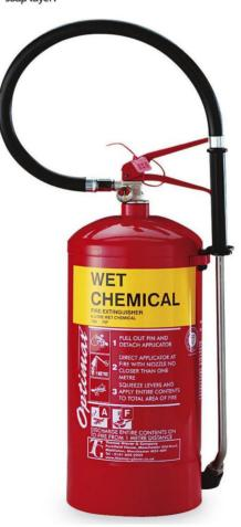
Some of the "foam based with special additive" extinguishers work by covering the hot burning oil with a thick heat resistant crust on top of the surface as above whilst at the same time cooling the burning oil by converting the extinguishing water into steam in a controlled manner.
